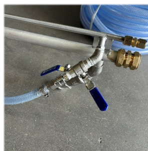
Air boost at bottom and top can be activated independent
